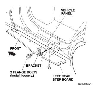
15. Loosely install the bracket to the vehicle panel with two flange bolts.
