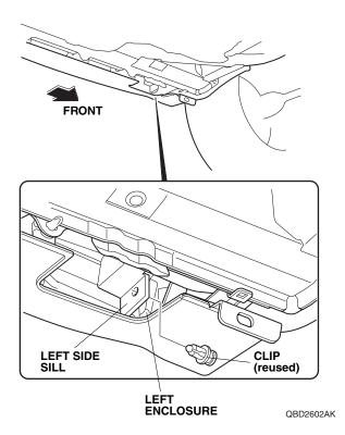
19. Secure the front of the left side sill with the one clip and two self-tapping screws removed in step 1.
