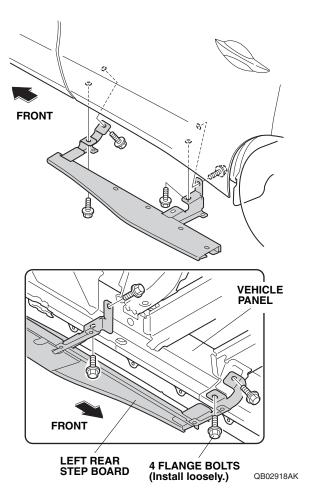
12. Loosely install the left rear step board to the vehicle panel using four flange bolts.
